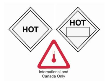
Figure 7. Elevated Temperature Material Mark
